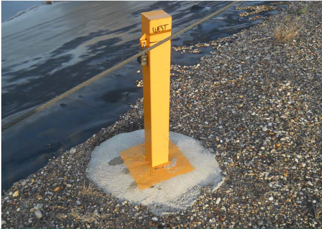
Photograph 5 (Center Cell) Piezometer on the east side of the Center Cell (DSCN0784.JPG)
