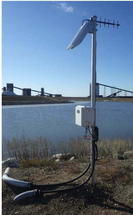
Photograph 8 (East/Center Cell berm crest) Pond level instrumentation panel (IMGP6347.JPG)
