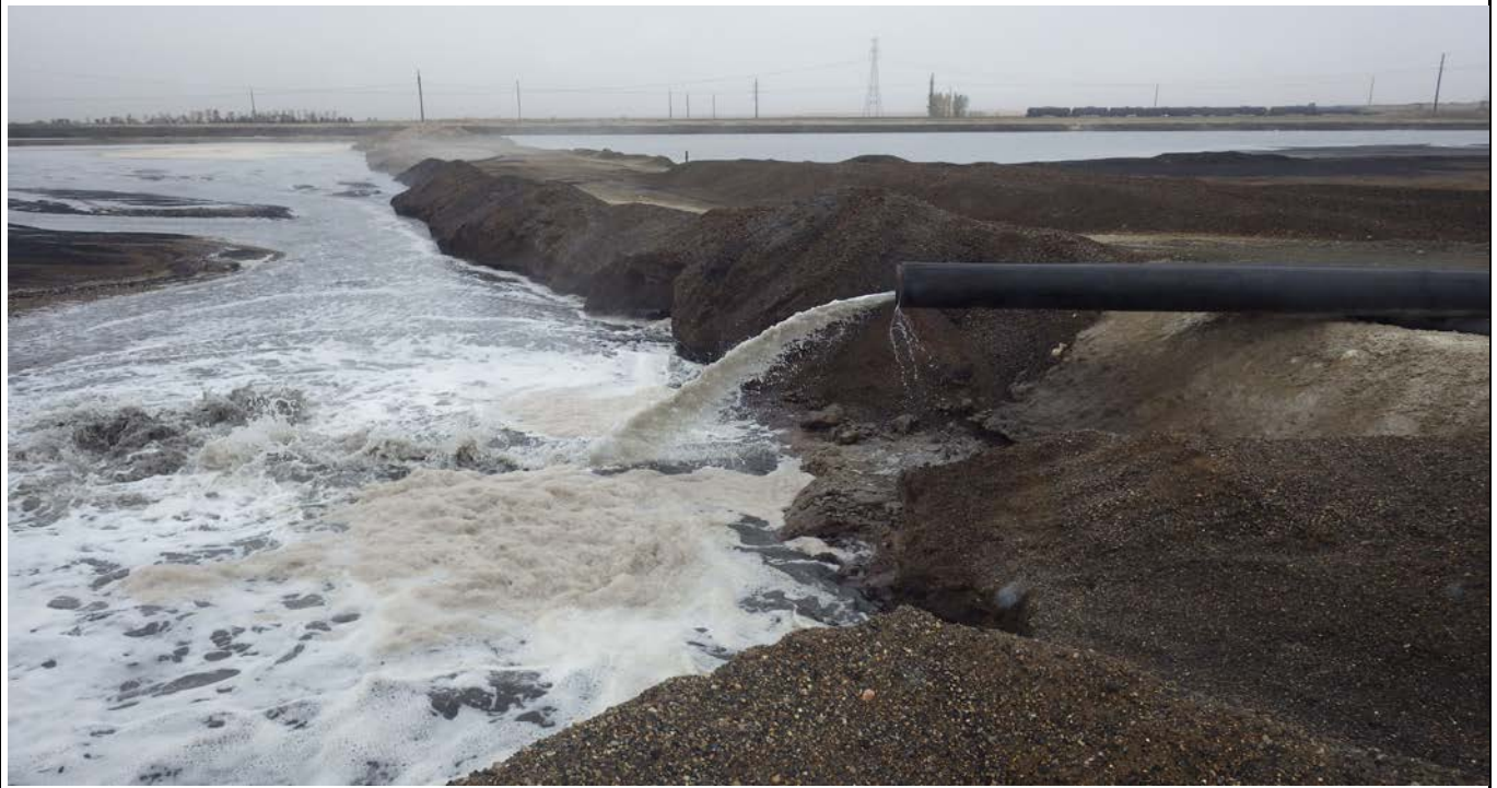
Photograph 7 (CCR placement) Rejects and economizer ash inflow pipe (IMGP6370.JPG)
