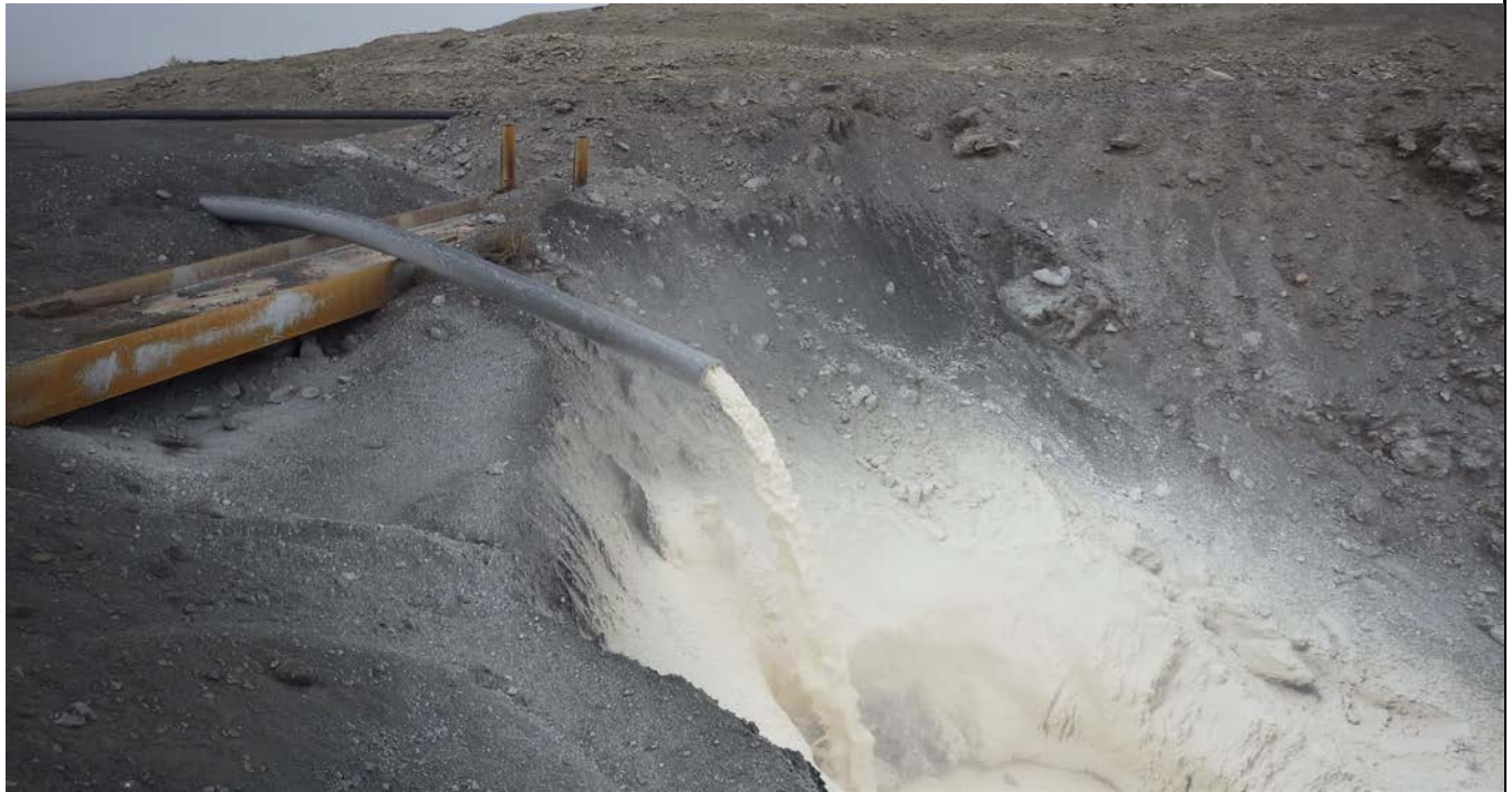
Photograph 4 (CCR placement) Flue Gas Desulfurization (FGD) inflow pipe (IMGP6366.JPG)
