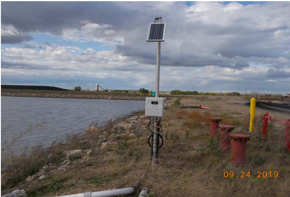
Photograph 19 (Center cell east berm crest) Water level monitoring station for center and east cells, good condition (PDS DPS (19).JPG)
