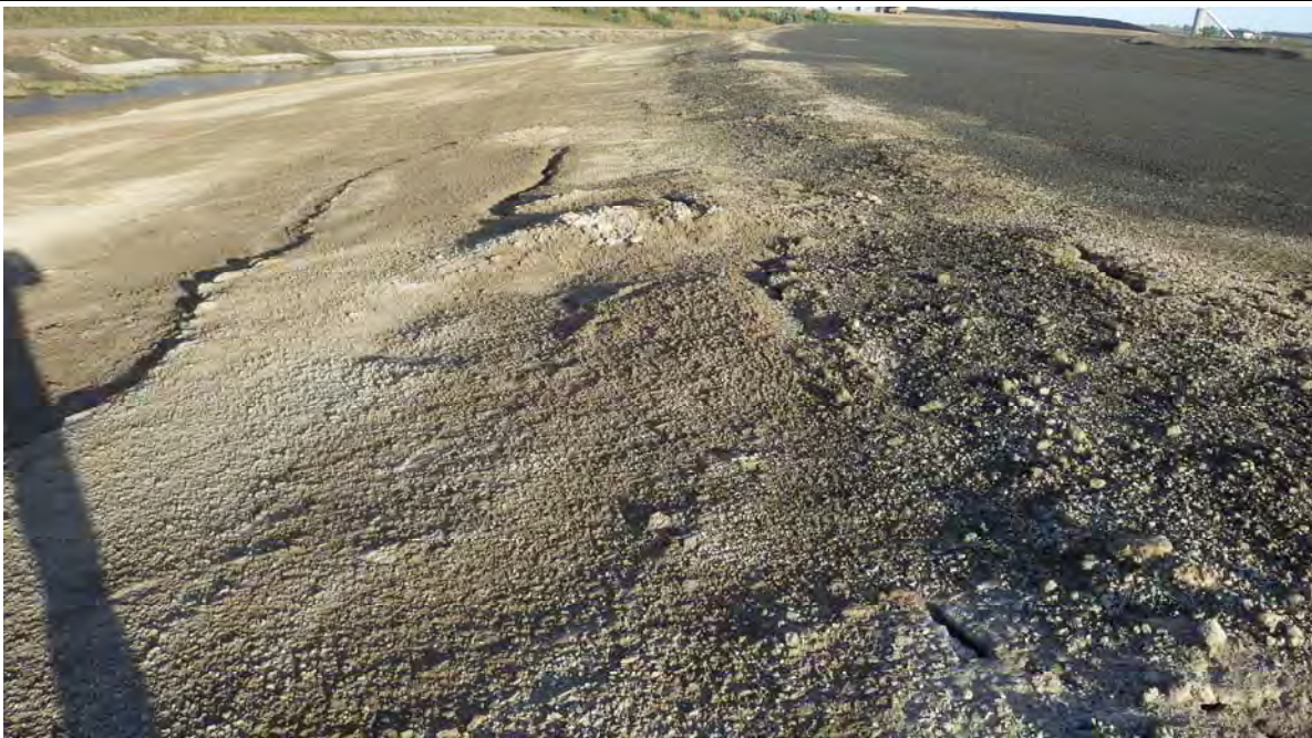
Photograph 8 (Southwest CCR downstream slope) Minor cracking of reactive fly ash on the CCR downstream slope (IMGP6982.JPG)
