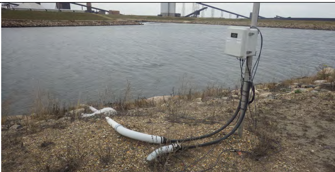
Photograph 20 (Center cell, west upstream slope) Center cell and east cell water level measurement station. (IMGP8079.JPG)
