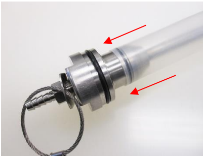
Figure 4-10a: Sliding bladder on
