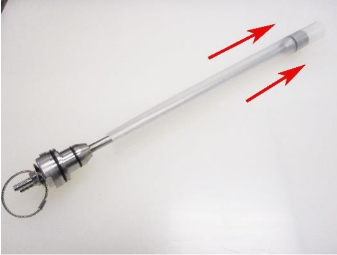
Figure 4-7: Removing the bladder
