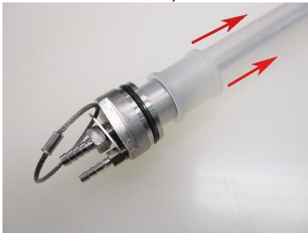
Figure 4-6: Removing upper compression ring
